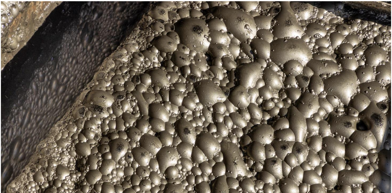
Figure 2 Copper concentrate production through the flotation circuit
