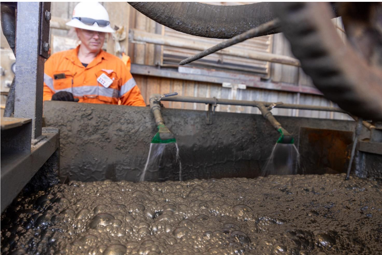
Figure 2 Copper concentrate production through the flotation circuit
